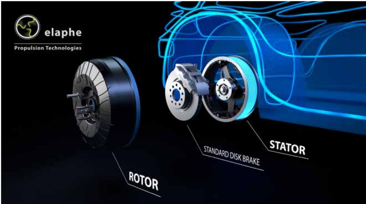
Elaphe's unique in-wheel architecture and control algorithms offer interesting advantages over traditional electric motors. Independent four-wheel drive minus mechanical transmission provides greater stability and responsiveness to road conditions.
