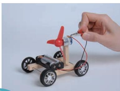
This propeller car reacts by moving forward whenever the propeller pushes the air backward. However, if the back of the car was blocked (as in the illustration below), what would happen?
