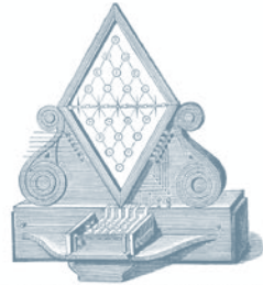
Fig. 750.—Cooke and Wheatstone's Five-Needle Telegraph.
