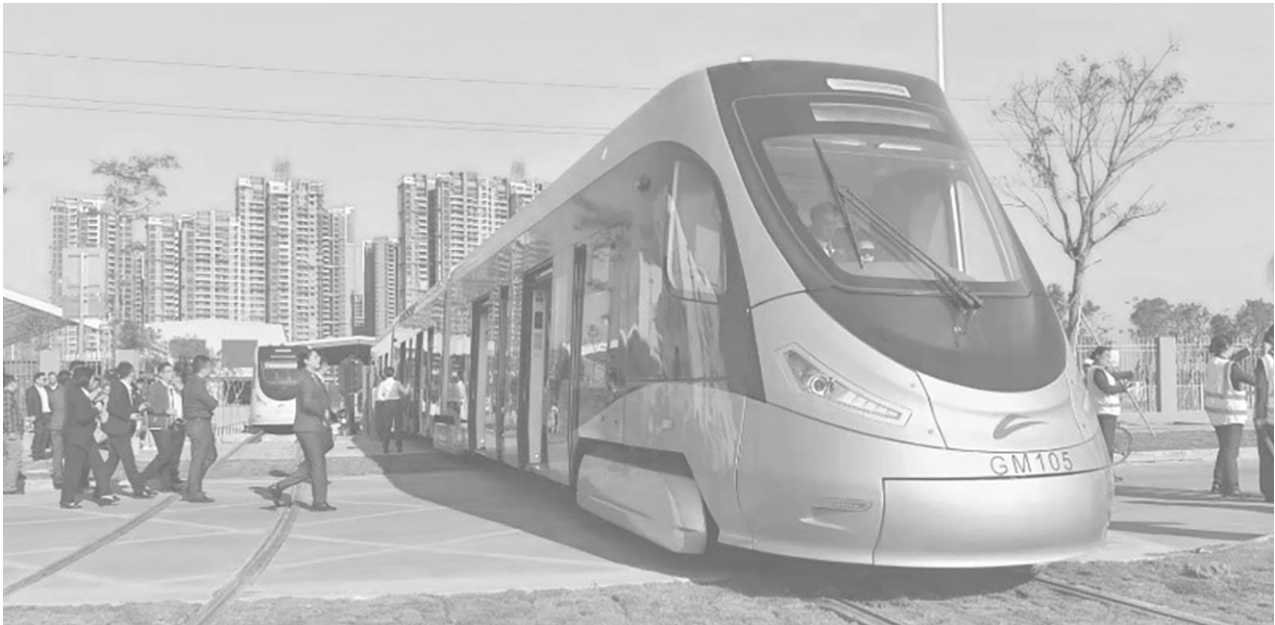
Hydrogen tram in Gaoming District, Foshan City (Guangzhou Daily, 2020).
