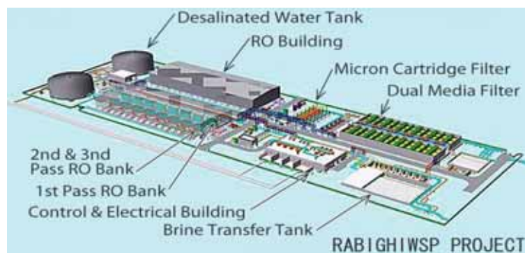
Figure 28: Plant schematic for a Mitsubishi-designed RO plant 14
