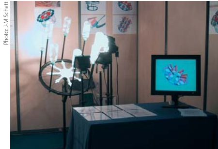
Jean-Marie Schatt's Thermoturbine prototype, ingeniously constructed from a bicycle wheel and bottles, produces rotary energy from thermal energy
