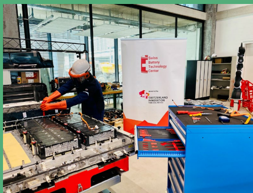
Battery Disassemble Operation at Swiss Innovation Park Biel/Bienne
