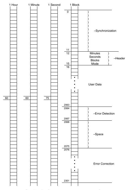
For 1 Hour, User Data = 60x60x75x2048=552,960,000 Bytes For 1 Hour, Total Data = 60x60x75x2352=635,040,000 Bytes
