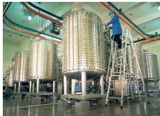
The Plafractor. Inventing a new fermentation system gave Biocon their technological and commercial breakthrough
