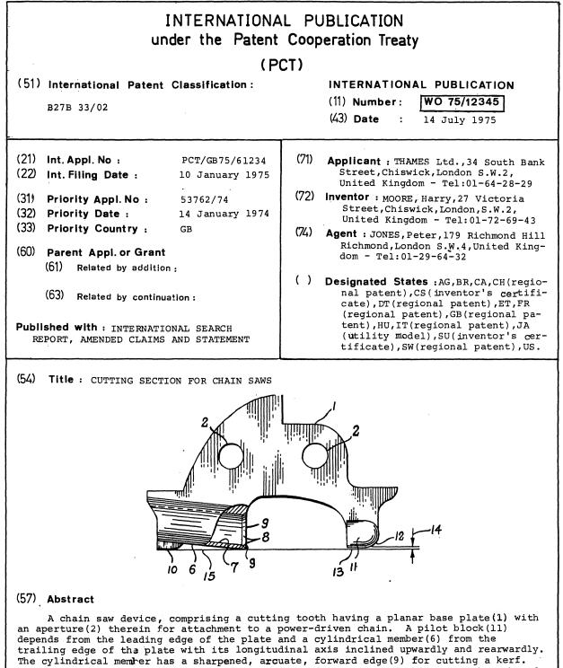
The cylindrical member has a sharpened, arcuate, forward edge(9) for cutting a kerf. A bore(7) extends through the cylindrical member for passage of chips therethrough and a heel portion(10) follows the forward cutting edge(9) for engaging and finishing the kerf. The chain saw device, while particularly designed for use in cutting wood, is also adapted for cutting minerals and other materials.
